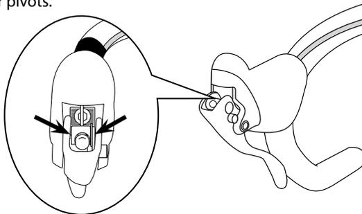
**IMPORTANT:** Cane Creek's Drop-V road brake levers are not designed to work with side-pull, center-pull, or cantilever brake calipers. Only linear-pull brake calipers designed for mountain, touring, or cyclocross riding can be used with this product.
