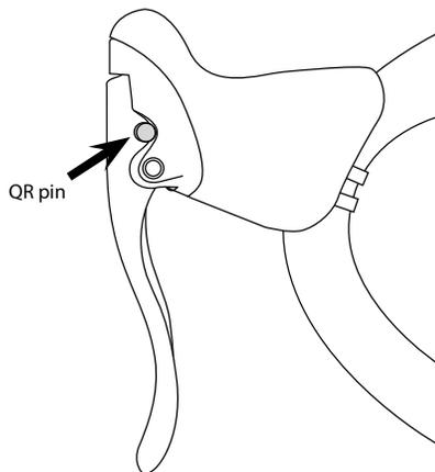
Fig. 4b - To reduce cable tension on the brake caliper for wheel removal, etc., press the cable QR pin fully AWAY from the handlebar stem.
