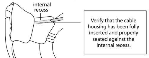
Fig. 3 - Secure the cable housing to the handlebar with electrical tape or a similar material.
